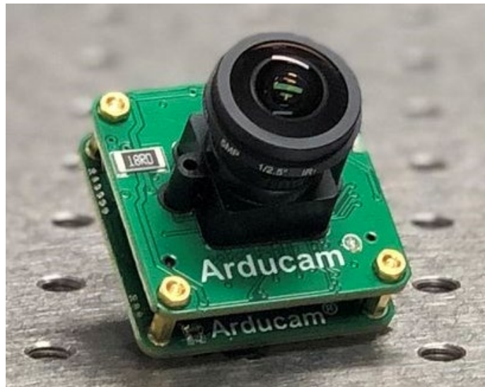
Figure 21: SKKU camera module (rev G) for use in both D-Eggs and mDOMs. The camera is common for both types of modules but a different mounting system is used for each type.
