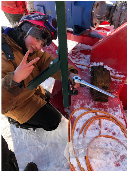
Figure 4. Lexi Oxborough working the Main Drill Hose Reel which is used for reeling and paying out the hose that carries hot pressurized water to the drillhead
