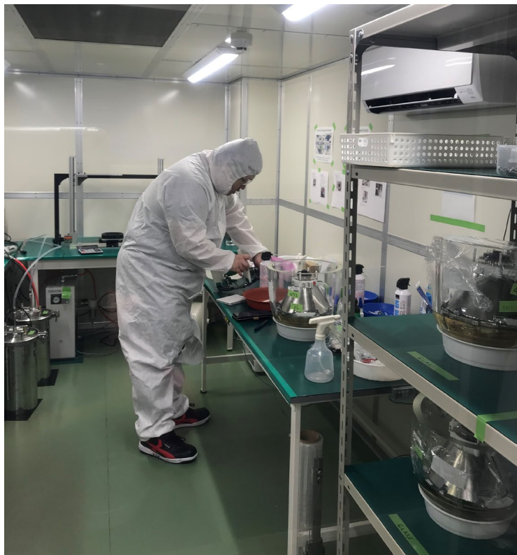
Figure 14: Cleanroom used in assembly and integration of D-Egg at the Nippon Marine Enterprises (NME) facility in Yokohama, Japan. Half D-Eggs here are being inspected and cleaned at this assembly step along the production line.
