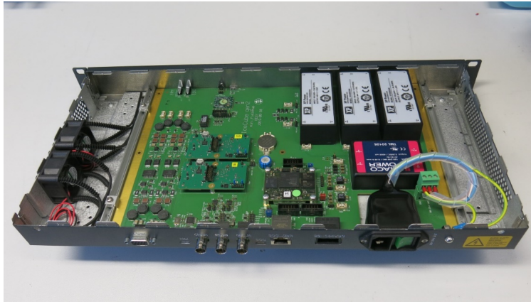
Figure 19: Mini-FieldHub (first version of readout electronics module). Mini-FieldHubs are used to communicate with DOMs and other sensors during sensor design verification testing, final acceptance testing of production sensors, and for software and firmware development. The mini-FieldHub design will evolve into the FieldHubs used to read out the deployed sensors from the ICL.
