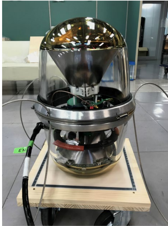
Figure 13: First of the D-Egg Design Verification Testing units, Chiba, January 2020. Ten modules were built and tested to verify the design met requirements before production was allowed to start.
