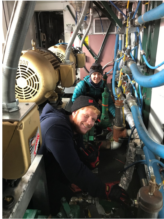
Figure 3. Barb Birrittella and Jake Nesbit working on high pressure pumps. The HPPs are used to pressurize the water that is sent through the main hose downhole to the drillhead.
