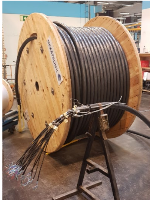
Figure 18: Downhole cable prototype ready for electrical testing. The downhole cable connects the optical modules, calibration devices and other devices in the ice to the surface cable at the surface junction box. There is one downhole cable for each hole.
