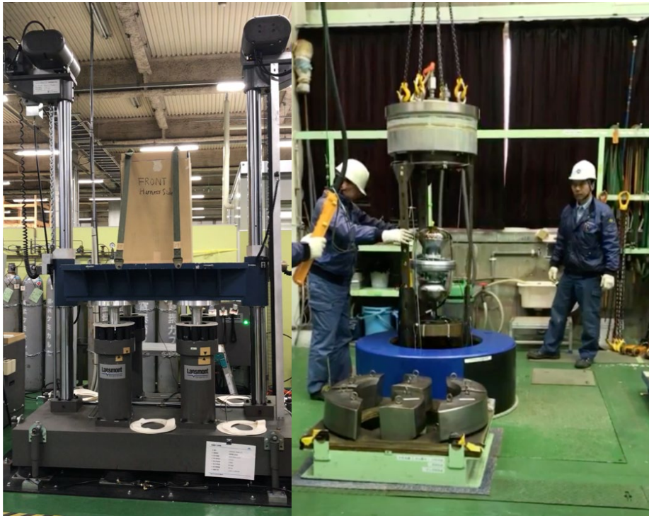
Figure 15: Integrated D-Egg design verification: industrial standard shock testing setup on the left and hydrostatic pressure testing to 10,000 psi (700 bar) on the right
